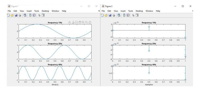
Based on the three sampled signals, can you figure out the original signals? Now, try to increase the sampling frequency to 4Hz. Can you figure out the original signals? How about further increasing the sampling frequency to 8 Hz? Can you explain why?
